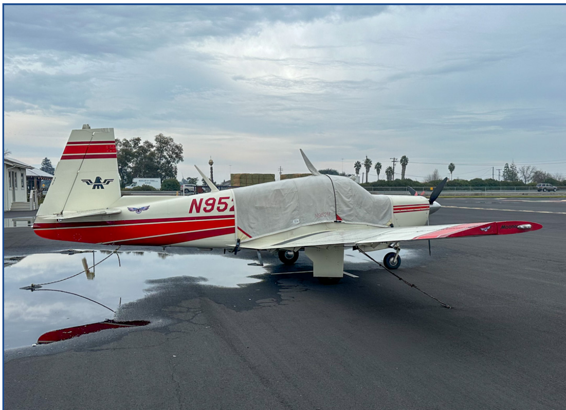
Mooney M20C Canopy Cover, extended to cover avionics panel.
