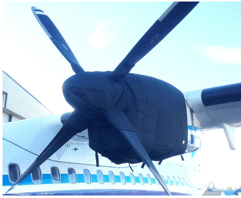
ATR-72-202 Insulated Engine & Prop Hub Covers
