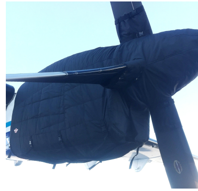
ATR-72-202 Insulated Engine & Prop Hub Covers
