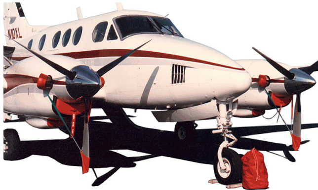
Pitot, Exhaust Covers, Engine Plugs & Prop Ties
