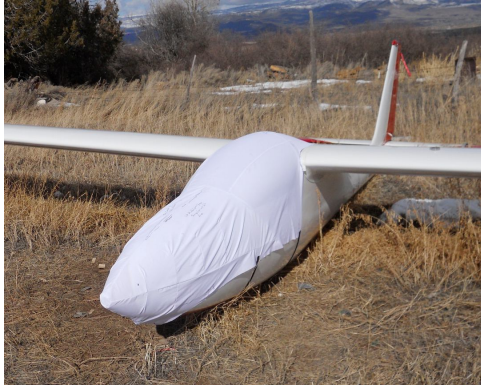
Laister LP-49 Canopy/Nose Cover, test fit cover
