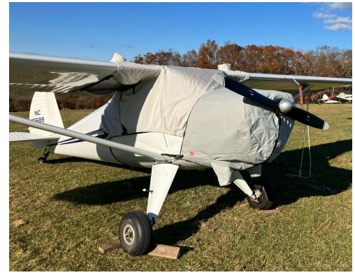
Luscombe 8E Canopy Cover w/Wing Extensions, Insulated Engine Cover Luscombe 8A Canopy Cover, Insulated Engine Cover
