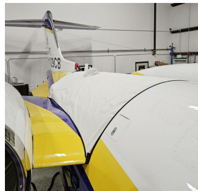
Lear 45 Empennage Saddle Cover W/ Dorsal Inlet Plug (Covers Upper Fuselage Between Pylons, Acm/Apu Area)
