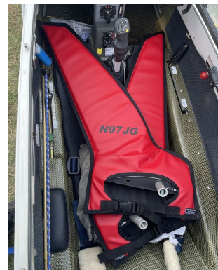
Schempp-Hirth Ventus-2B winglet/wingtip pads
