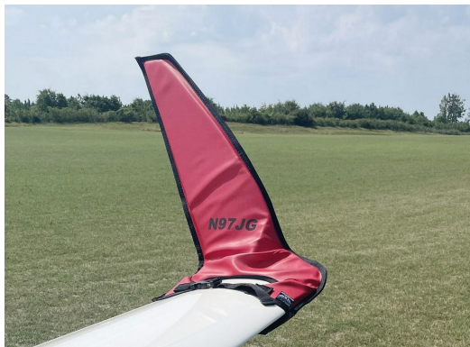
Schempp-Hirth Ventus-2B winglet/wingtip pads
