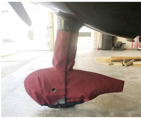
Cessna Corvalis, Lancair Columbia Wheelpant & Strut Cover
