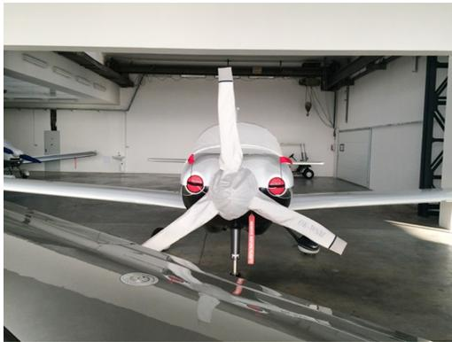
Cessna 350/400 Engine Inlet Plugs, 3-Blade Prop Cover
