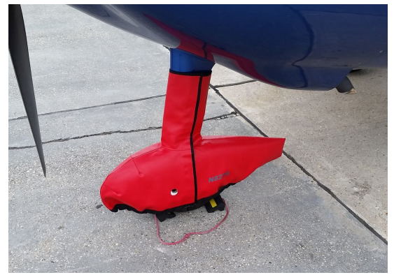
Lancair Columbia Nose Wheelpant/Strut Cover
