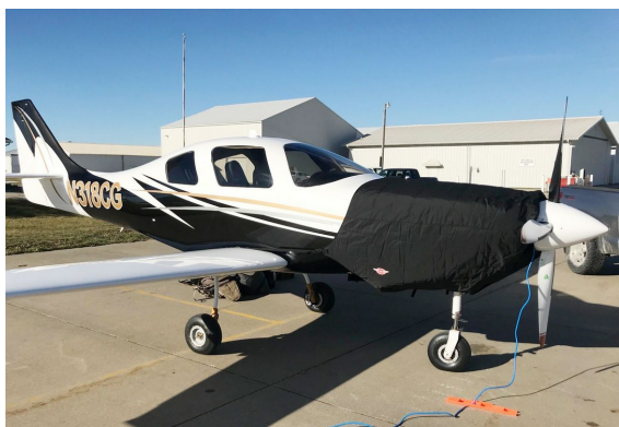
Lancair IV-P Insulated Engine Cover, fully enclosed
