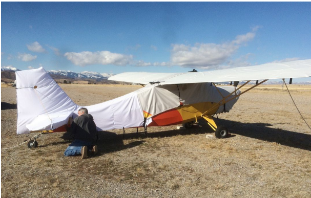
Aeronca Champ Canopy, Wings, Engine & Empennage (test fit) Covers
