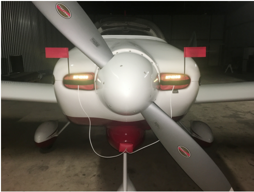
Van's Aircraft RV-7A Engine Inlet Plugs ENGINE PLUGS PREVENT BIRD NEST FOD. Piper Saratoga Engine Cowling Bird's Nest
