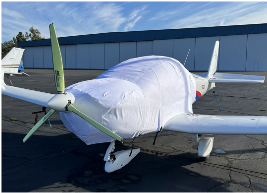
Jihlavan JA-600 Skyleader Extended Canopy/Engine Cover, test fit cover
