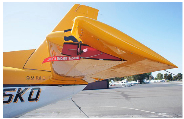
Quest Kodiak Horizontal Stabilizer Lightning Hole Plugs
