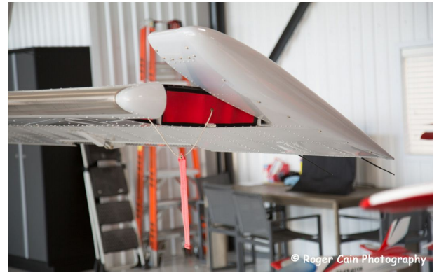
Quest Kodiak Horizontal Stabilizer Lightning Holes Plugs
