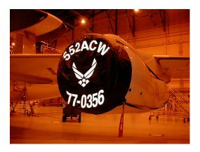
Intake/Exhaust Covers, soft type, TF-33 Engines
