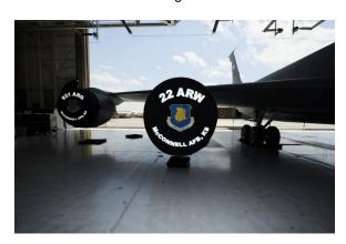
KC135 Intake Covers, Soft Type, R-Model, CFM56 Engines
