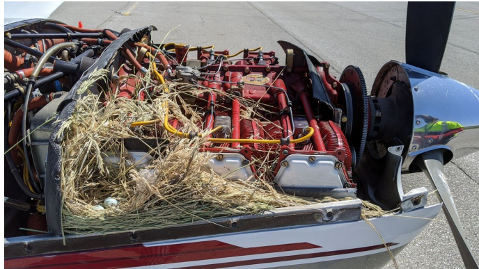
Preceptor STOL King Engine Plugs ENGINE PLUGS PREVENT BIRD NEST FOD. Piper Saratoga Engine Cowling Bird's Nest
