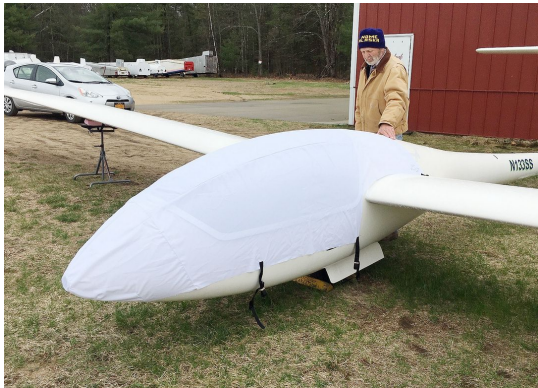
Grob 102 Astir CS Canopy/Nose Cover (test fit)
