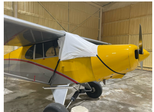
Piper J5A Windshield/Skylight Cover, test fit
