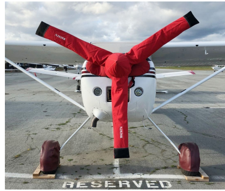
Cessna Skywagon Propellor/Spinner Cover, 3-blade type
