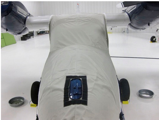
Grumman Widgeon Cockpit/Nose Cover, tie-down cleat detail
