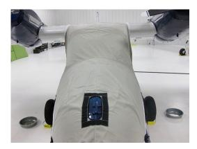
Grumman HU-16 Albatross Cockpit/Nose Cover and Engine Cover(test fit Grumman Widgeon Cockpit/Nose Cover, tie-down cleat covers)
