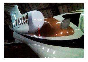
Phenom 100 Intake/Exhaust Cover, "Bikini" Type
