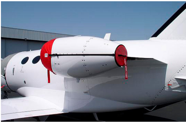
Cessna Mustang Intake/Exhaust Plug Set
