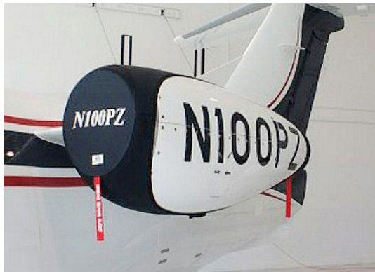
Phenom 100 "Bikini" Engine Covers
