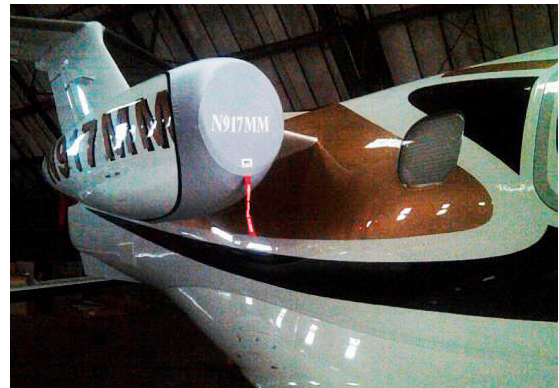
Phenom 100 Intake/Exhaust Cover, "Bikini" Type
