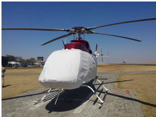
Bell 407 Bubble Cover with Wire Strike
