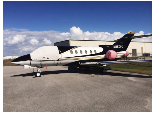
Hawker 800 Cockpit Cover, extended aft 24"
