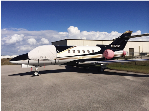
Hawker 800 Cockpit Cover, extended aft 24"
