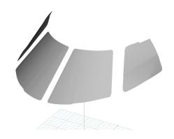
Gulfstream G150 Cockpit HeatShields (3D Model)
