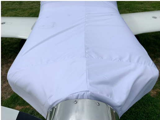
Grob 115 Canopy/Engine Cover, test fit cover
