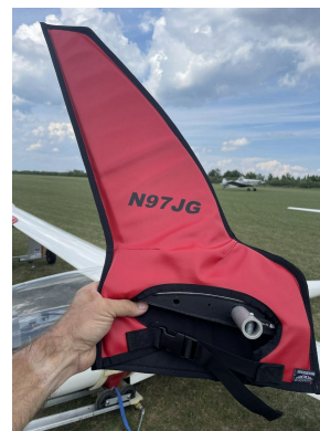
Schempp-Hirth Ventus-2B winglet/wingtip pads
