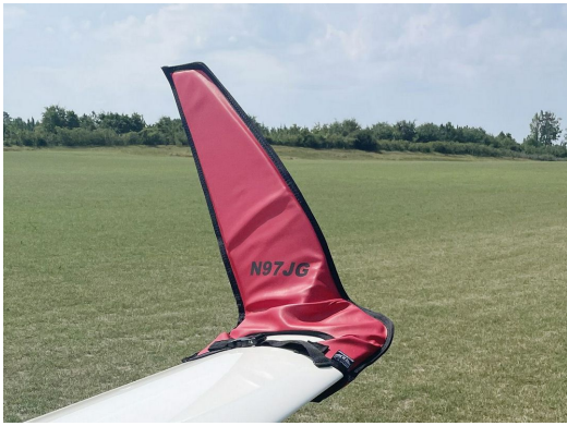
Schempp-Hirth Ventus-2B winglet/wingtip pads
