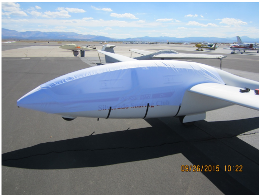
DG-505 Canopy/Nose Cover (test fit cover)
