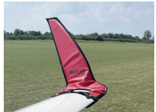
Schempp-Hirth Ventus-2B winglet/wingtip pads
