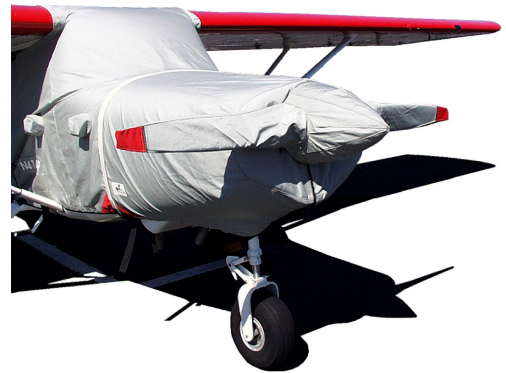
Maule Prop (2 Blade), Engine, & Canopy Cover
