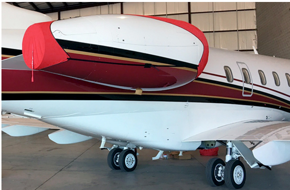
Intake/Exhaust Covers, 3-Strap Type. Successfully installed by two crew, one ladder. Falcon 6X Engine Cover, 3-Strap Type
