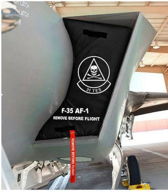
Joint Strike Fighter F-35 Engine Intake PLUG ASSY
