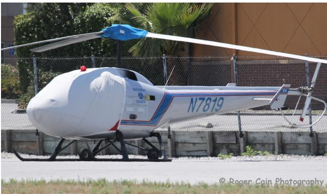
Enstrom 280FX Bubble Cover, Rotor Mast Cover
