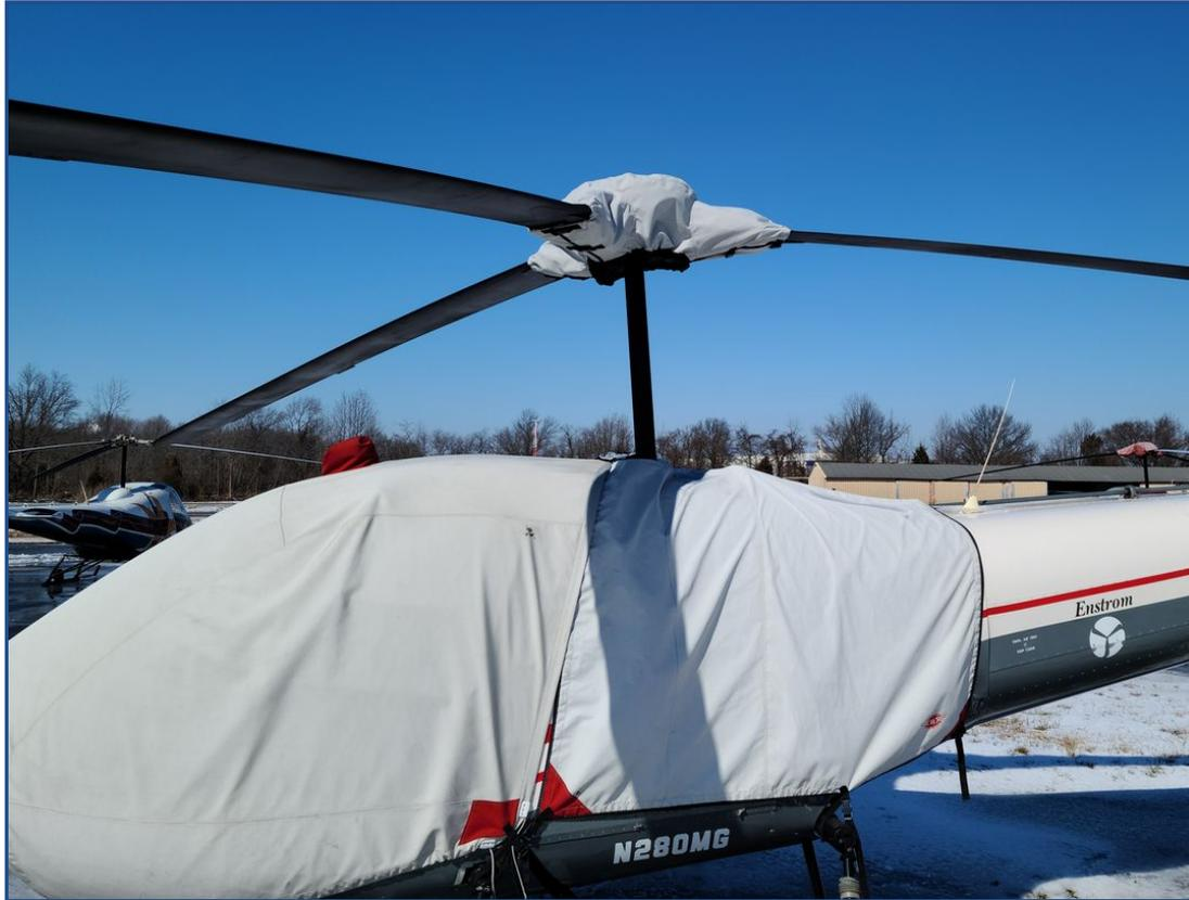
Enstrom 280C Shark Bubble, Engine & Rotor Hub Covers
