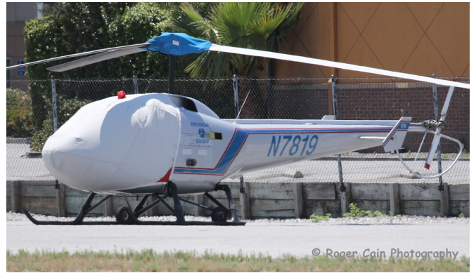
Enstrom 280FX Bubble Cover, Rotor Mast Cover
