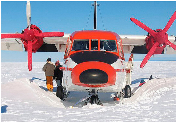
Casa 212 Insulated Engine & Propellor/Spinner Covers
