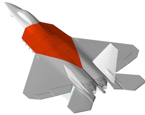
Boeing 757 Tire Covers, Wash Down or Long-term Storage Lockheed F-22 Raptor Upper Surface Rain Barrier Cover, 3D model
