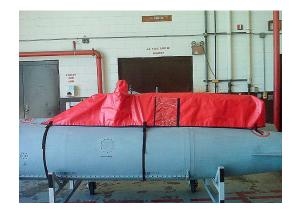
370 gal. WING FUEL TANK PYLON COVER, with/without forms pouch
