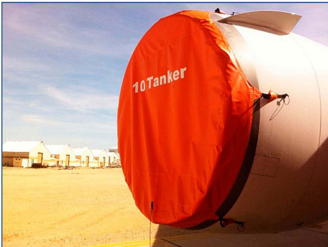
DC-10-30 Intake Cover (CF650C2 Engine)
