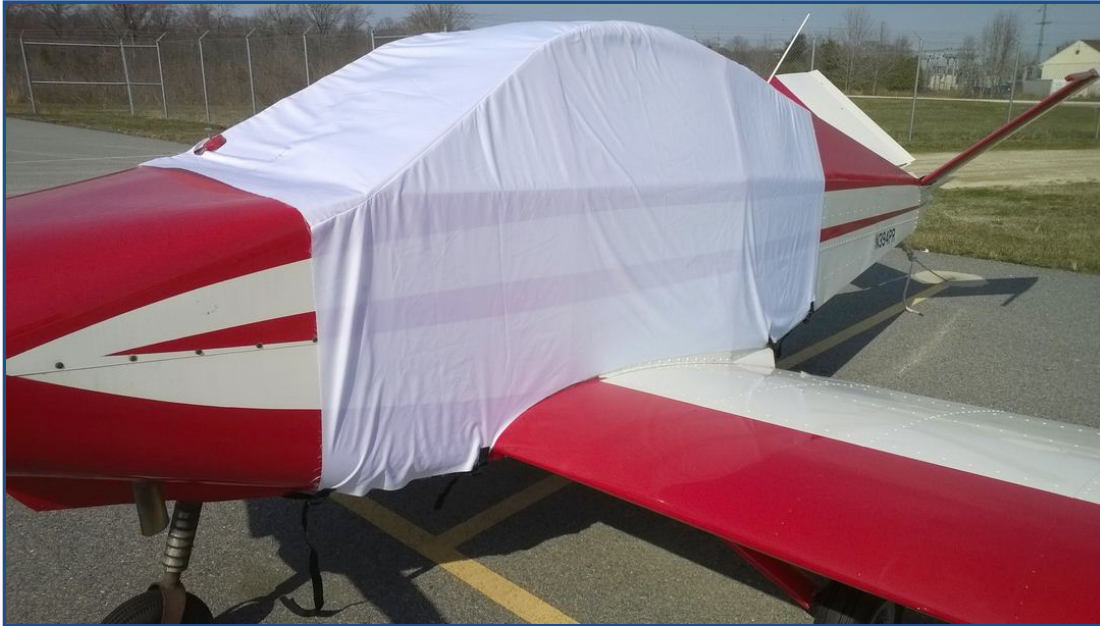
Davis DA-2A Extended Canopy Cover, test fit cover
