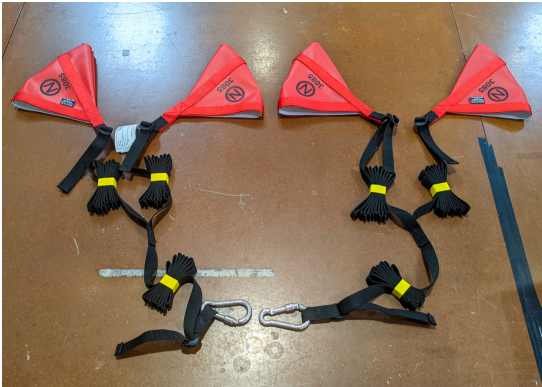
Dornier 328 Turboprop, C-146A Wolfhound Prop-Tie Downs, Turbo Prop Engines
