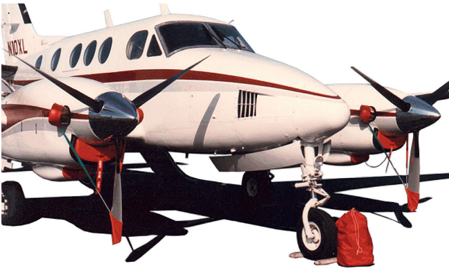
Pitot, Exhaust Covers, Engine Plugs & Prop Ties
