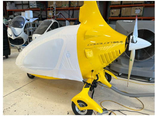
Autogyro Cavalon Canopy/Nose Cover, test fit cover
