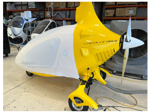
Autogyro Cavalon Canopy/Nose Cover, test fit cover
