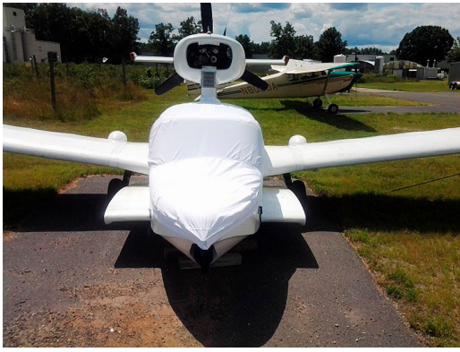
Taylor Coot Canopy/Nose Cover, test fit cover
