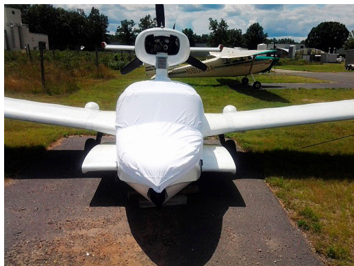
Taylor Coot Canopy/Nose Cover, test fit cover
