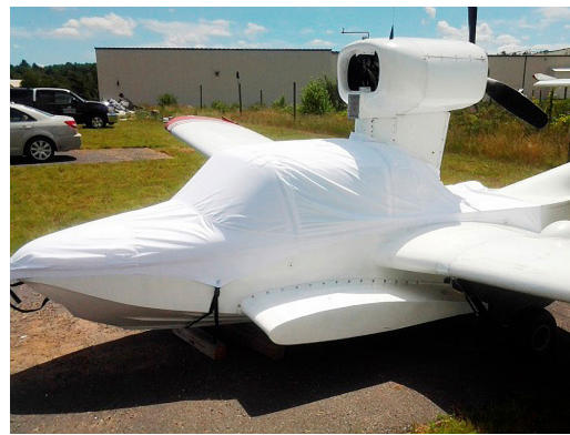
Taylor Coot Canopy/Nose Cover, test fit cover
