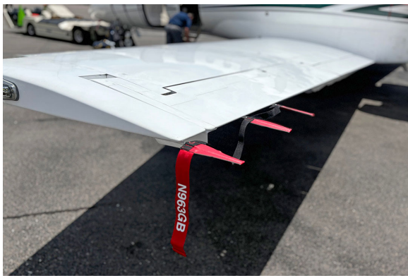
Cessna Citationjet 525C, CJ-4 Static Wick Protectors, 3 Per Wing, 1 On Tailcone Area
