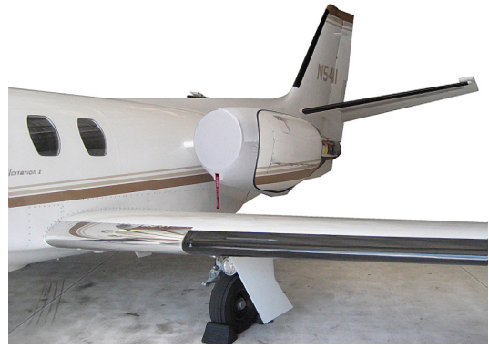
Cessna Citation "Bikini" Type Engine Covers: Extremely Light & Portable
