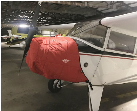
Piper PA-15 Vagabond Insulated Engine Cover
