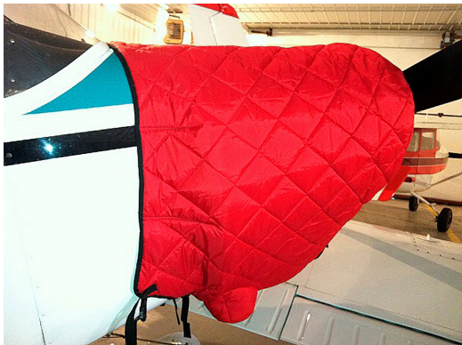
Piper PA-18 Super Cub Insulated Engine Cover
