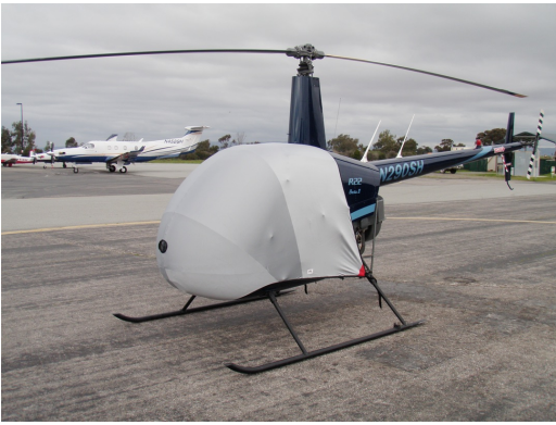
Robinson R-22 Light Weight Travel Cover Robinson R-22 Bubble Cover (Ext. Past Rotor Hub), Engine Cover, Tailboom Cover, Blade Covers, Rotor Hub Cover, & Tail Rotor Gear Box Cover
