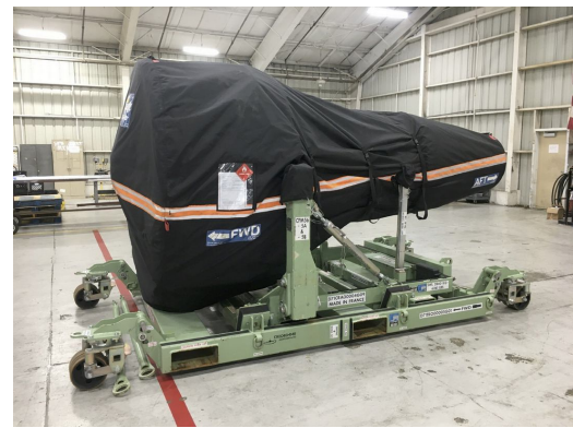
CFM56-5B Off Link Cover, fully enclosed
