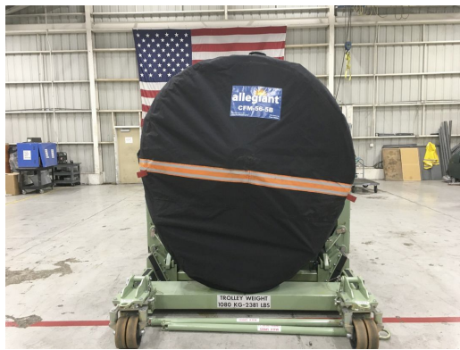
CFM56-5B Off Link Cover, fully enclosed
