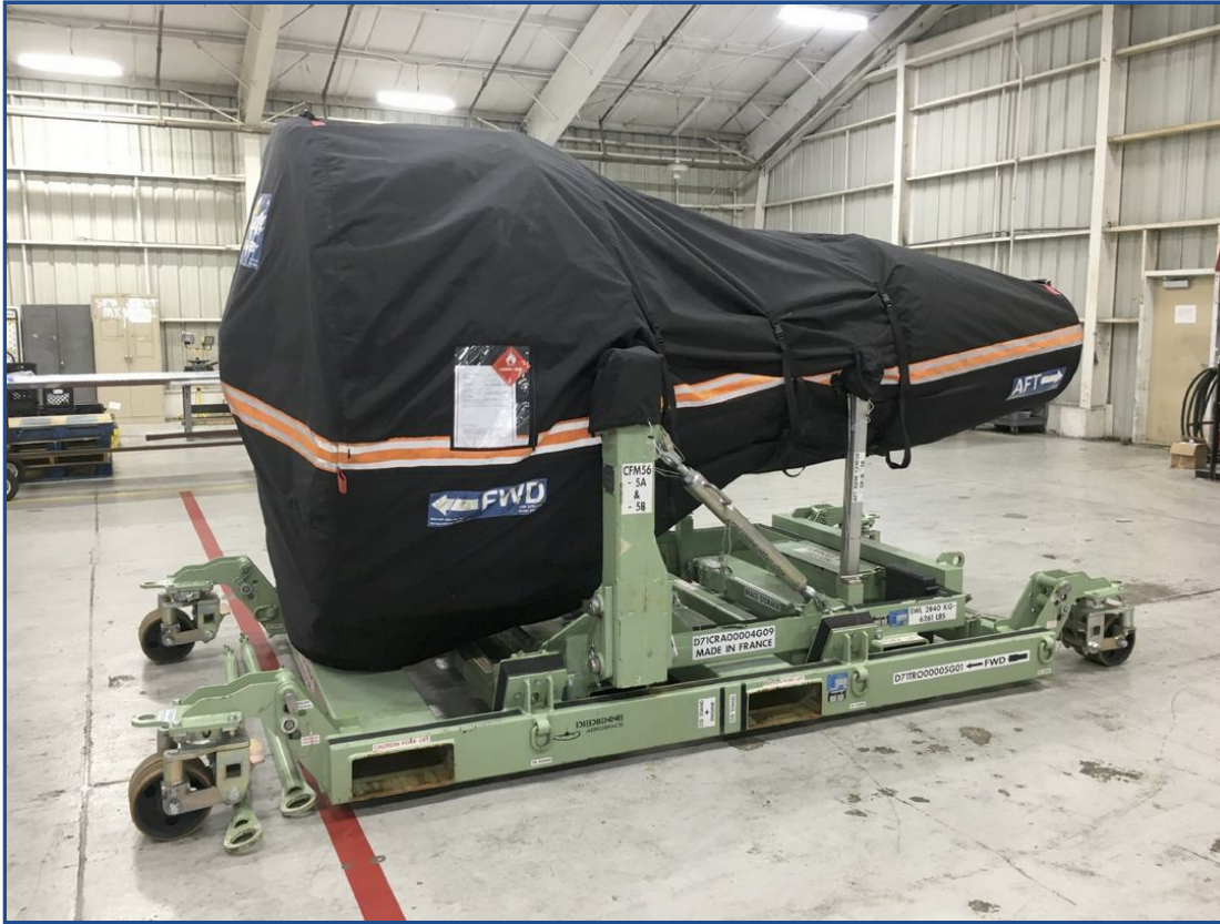
CFM56-5B Off Link Cover, fully enclosed
