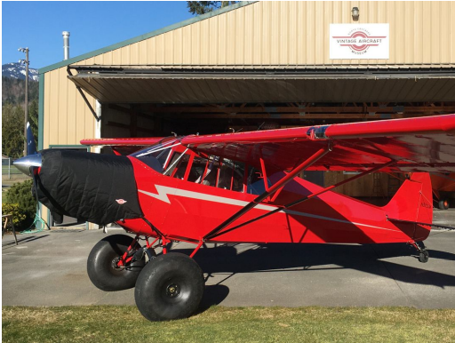
Piper PA-12 Insulated Engine Cover
