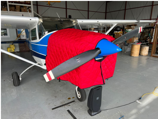
Insulated Hangar Blanket on Cessna 182
