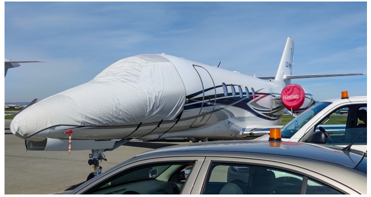
Cessna Citation Latitude (680A) Cockpit/Nose Cover, Doesn't Cover Pitot Tubes
