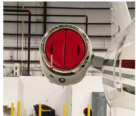
Embraer Legacy 500 Engine Inlet Plugs, folding type
