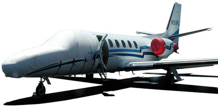
Cessna Citation Nose/Cockpit Cover, Engine Covers
