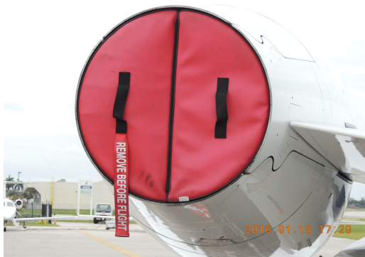
Embraer Legacy 500 Engine Exhaust Plug, folding type
