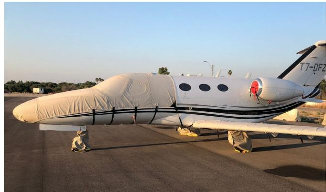
Cessna 510 Mustang Cockpit/Nose Cover, Engine Inlet Plugs
