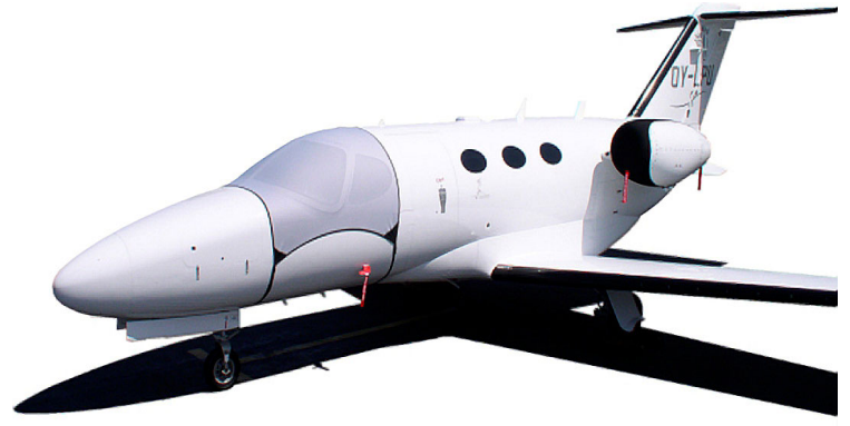
Citation Mustang Light Weight Travel Windshield Cover, "Bikini" type Engine Cover Set
