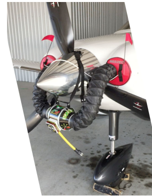
TTx Plugs for Aerotherm Preheater
