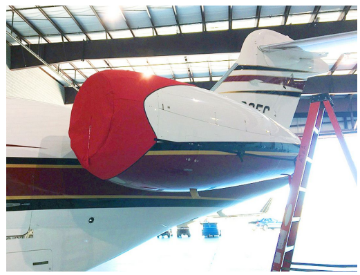
Canadair Challenger 300 Intake/Exhaust Covers, 3-Strap Type
